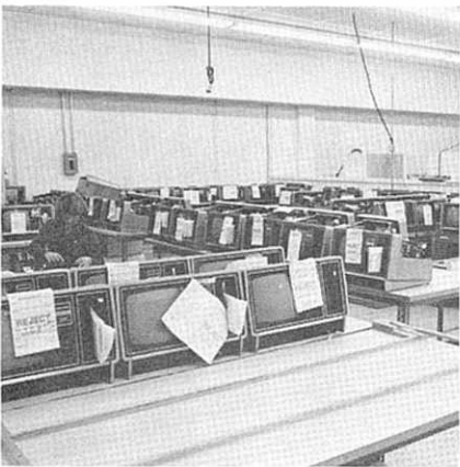
Any unit showing any problems or instability is rejected and sent back for further checking and repairs. They are very picky.
